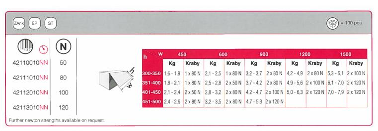
The above chart refers to chipboard or MDF 18 mm doors and aluminium frame doors with glass 4 mm thick
