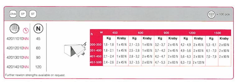
The above chart refers to chipboard or MDF 18 mm doors and aluminium frame doors with glass 4 mm thick. These are experimental results to be checked by the customer.
