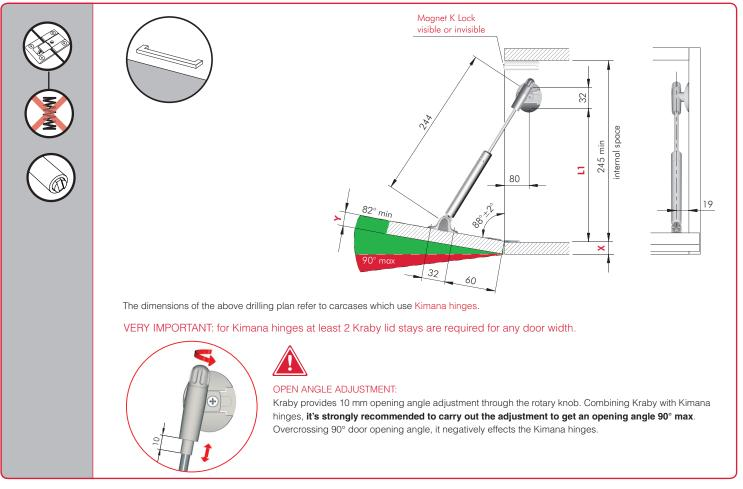
For pistons quantity to be specified according to door size, refer to the chart for "KRABY 244 mm - DROP DOWN".
